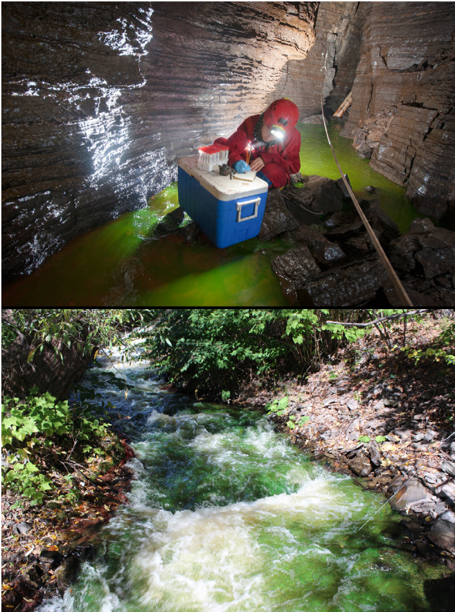
Fig. 6. Water sampling in an accessible cave during the fluorescein dye tracer test (top - site 1 on Fig. 1) and at a spring (bottom - site 4 on Fig. 1). (Top picture by Guillaume Pelletier.)
