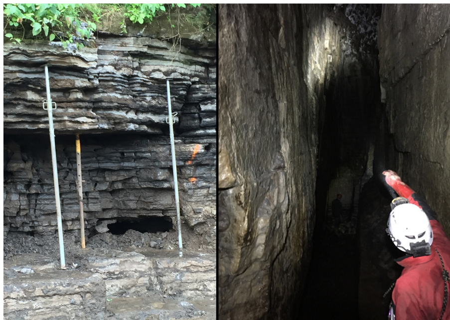
Fig. 2. Example of an infiltration hole along the Montmorency River bank at the dam observable after decreasing the water level (left picture; see inflow location on Fig. 1) and view inside an accessible section of a cave (see point 2 on Fig. 1).
